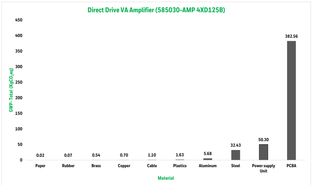
Figure 2 GWP – Total (A1) kg CO 2 e of materials used in Direct Drive VA Amplifier (585030-AMP 4XD125B)
