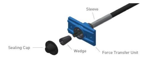
The XU2 system covers the whole anchor assembly comprising the coated steel force transfer unit, the steel wedge, the plastic sleeve, the plastic nut and the plastic sealing cap.
