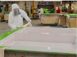
Thirdly and once semi cured, the gelcoat facing is backed up with a glass fibre reinforcement impregnated with a catalysed polyester resin. Immediately after application, the glass fibre and resin mix are consolidated and pressed onto the gel coat finish to which it chemically bonds to form a single composite panel.
