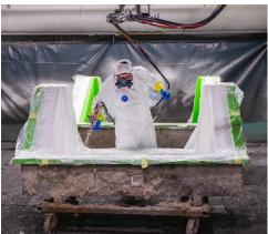
Thirdly and once semi cured, the gelcoat facing is backed up with a glass fibre reinforcement impregnated with a catalysed polyester resin. Immediately after application, the glass fibre and resin mix are consolidated and pressed onto the gel coat finish to which it chemically bonds to form a single composite panel.
