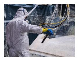
The parts are left to cure and once all elements have competed the curing cycle, the parts are released from the mould. The mould is then cleaned and prepared for repeating the process. These GRP parts, along with structural framing and insulation are assembled and fixed together to produce the final product. An insulated spray foam is sprayed into the void.
