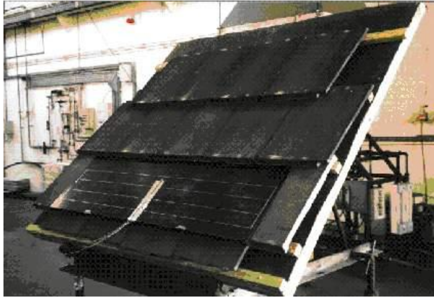
Figure: A2.1 A typical PV system ready for testing to BS 476-3 2004.
